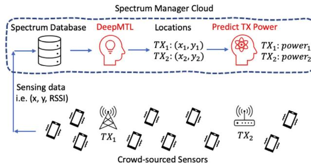
**Fig. 1.** Multiple transmitter localization using a distributed set of sensors. Sensing data is uploaded to a spectrum manager server in the cloud. DeepMTL is a deep learning approach to multiple transmitter localization which helps protect spectrum against unauthorized usage. After that, prediction of transmission powers happens using DeepMTL as a building block.
