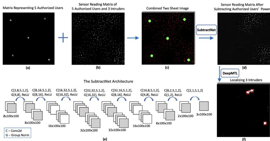
**Fig. 8.** Overall architecture of second approach to localize 3 intruders in the presence of 5 authorized users. The input of the SubtractNet is (c), which is stacking authorized user matrix (a) and the sensor reading matrix (b). (d) is the output of SubtractNet, where the transmission power of the authorized users is subtracted from the area. The details of the SubtractNet model is in (e). (f) is the localization output after feeding (d) into DeepMTL.
