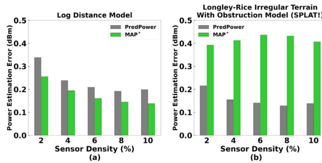
**Fig. 23.** The single transmitter power estimation error of PredPower and MAP\* in two propagation models, (a) Log-distance model and (b) Longley-Rice Irregular Terrain with Obstruction Model (SPLAT!), for varying sensor densities.
