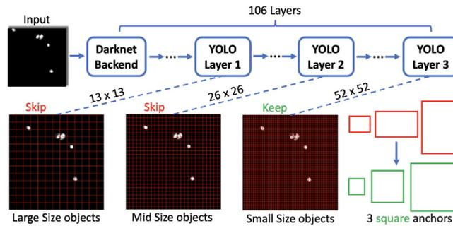
**Fig. 5.** Our YOLOv3-cust in the second step of the DeepMTL. The two major customization are: (i) Use only the third YOLO layer that detects small size objects (the output of YOLOv3-cust is the bounding box predicted by the third YOLO layer and we use the center of the bounding box as the transmitter location), and (ii) change the rectangle anchors to square anchors.
