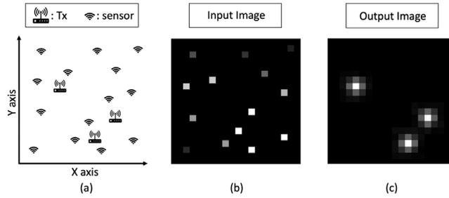
**Fig. 3.** Illustration of DeepMTL first step's input and output images. (a) Area with distributed sensors and transmitters to be localized. (b) Input image representing the sensor readings (RSS) and locations. (c) Output Image, where we put a 2D Gaussian distribution with its "peak" at the transmitter's location.
