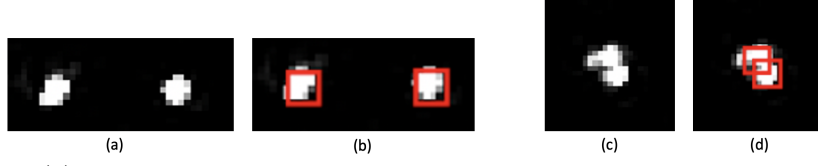
FIGURE 3.6: (a) is the zoom-in of two peaks at the bottom of the Fig. 3.2 example. (c) is the zoom-in of the two close by peaks in the middle right of the Fig. 3.2 example. (b) and (d) shows the bounding boxes that YOLOv3-cust outputs for (a) and (c) respectively.
