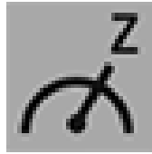
FIGURE 6.1: The only measurement gate provided by the IBM Quantum Computer is a measurement in the standard basis, also known as the z basis or computational basis. It can be used to implement any kind of measurement when combined with other gates.
